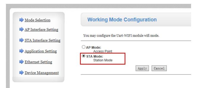
4. From the left hand menu select STA Interface Settings. Set the AP's SSID to your local WIFI network along with the security type and pass phrase. In the WAN connection drop dropdown select STATIC (fixed IP) and complete the form with the IP address assigned for your USR controller Click on Apply but do not restart the system
