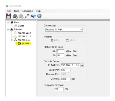
15. You can use this Utility to turn on / off the Digital Outputs (relays) by clicking on the ICON as shown below.
