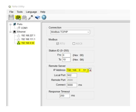
14. If successful the Controller will be listed under the Network. Click on this ICON to control the controller. Please note that you cannot change configuration settings in this mode. These can only be changed via the COM port.
