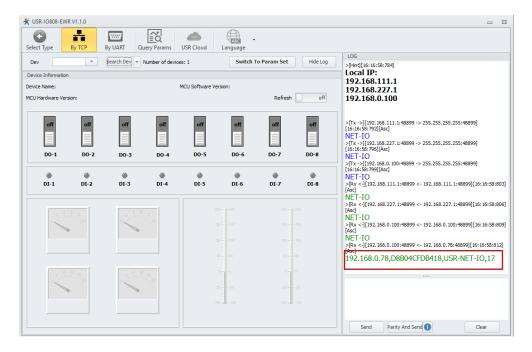
Next click on the **Dev** drop down and select the USR controller. You can now turn on or off any of the replays using the graphical interface.
